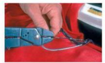
P14-3 Cut out the damaged wire.
