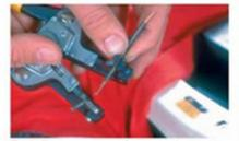
P14-5 Now remove about 1/2 inch of the insulation from both ends of the replacement wire. The length of the replacement wire should be slightly longer than the length of the wire removed.
